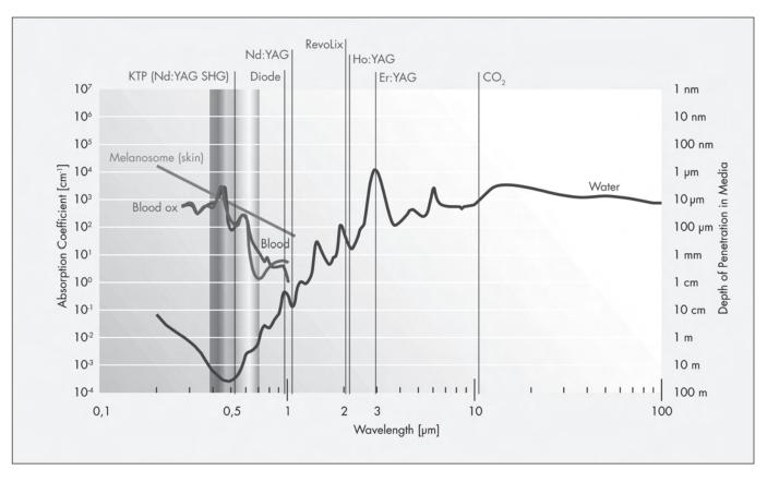
wave **RevoLix**<sup>TM</sup> laser has a wavelength of  $\lambda$ =2013 and the target chromophore is water. It is a full contact laser and employs a forward firing fiber for precise delivery of the laser energy. The fiber is reusable and therefore cost effective—about \$75 per procedure. The tissue can be vaporized or resected for histology. There is no concern of injuring unintended structures because the energy is absorbed within 1.0 mm from tip of the fiber in the irrigant.
